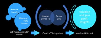
Collating the data via a cloud ingestion framework, generative AI is used to derive insights into the inverters, including the ability to identify outliers and usage trends.
